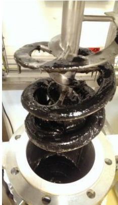
Dissolution of cellulose + carbon nanotubes in H_3PO_4 in a 10L reactor
