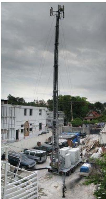
Figure 101 – Antenne mobile autonome
