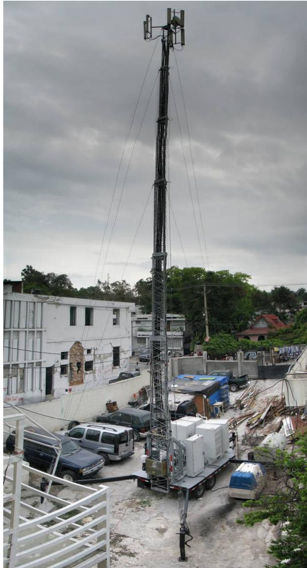
Figure 215 - Antenne mobile
